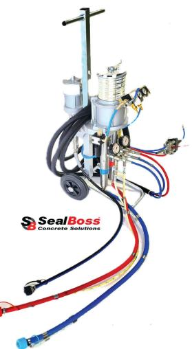
This complete package includes the stainless steel applicator with static mixer, a 15' triple set of high pressure hoses, triple set of suction hoses. The individual components are pumped separately and mixed in the mix head of the applicator while pumped through a plastic disposable element. Check valves prevent the components from cross contamination.
